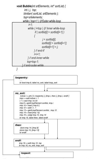
Figure 1: Bubble sort code fragment and intermediate code corresponding to inner loop
