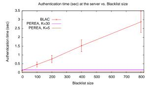
(a) The authentication time at the SP grows linearly with blacklist size for BLAC. The error bars represent one standard deviation. The authentication time for PEREA is constant; the two horizontal bands represent one standard around the means.
