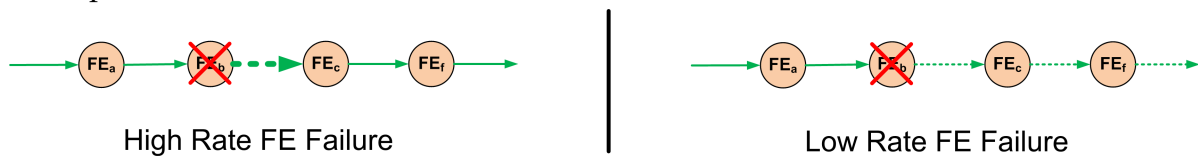
Figure 5.3. Left: an example of a high rate failure not being forwarded. Right: an example of a low rate failure being propagated to the next FE.
