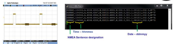
Garmin 18x LVC GPS timing pulse (left) which marks the start of each second has a data within the signal (right). The date and time data extracted for the synchro-phasor data time stamp, read by Putty terminal, is highlighted.
