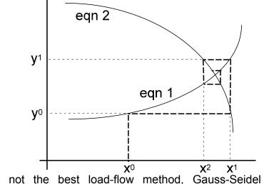
Although not the best load-flow method, Gauss-Seidel is the easiest to understand and was the most widely used technique until the early 1970s.
