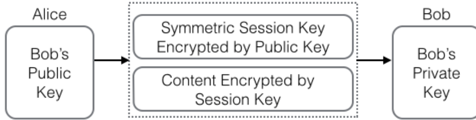
Figure 3.2: Encryption Scheme Used in CryptVMI
